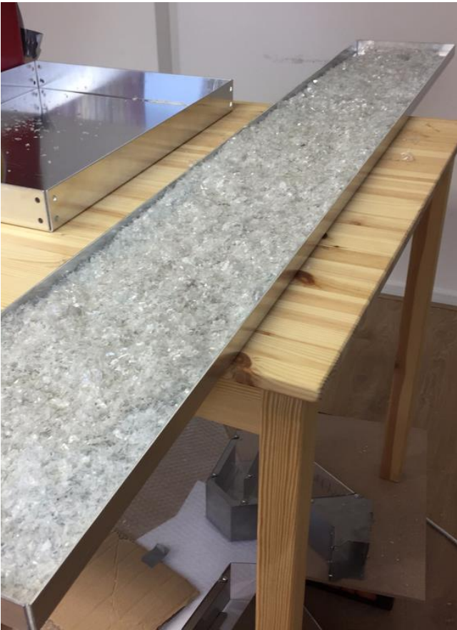
Figure 8: Dried PET regrind
