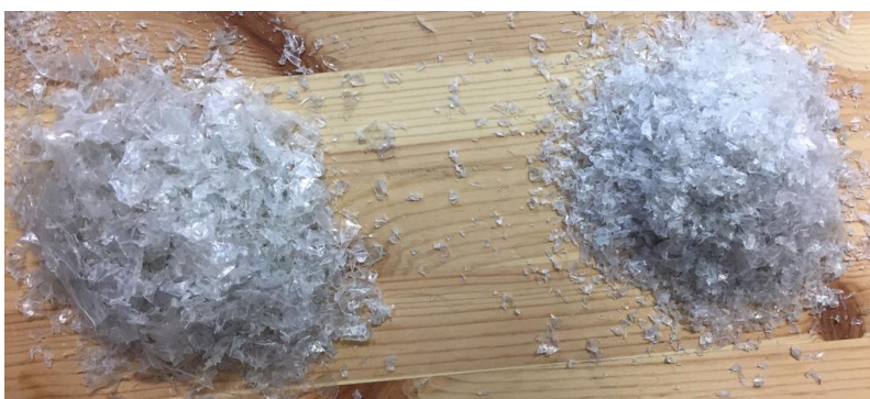
Figure 7: PET regrind and reshredded PET regrind
