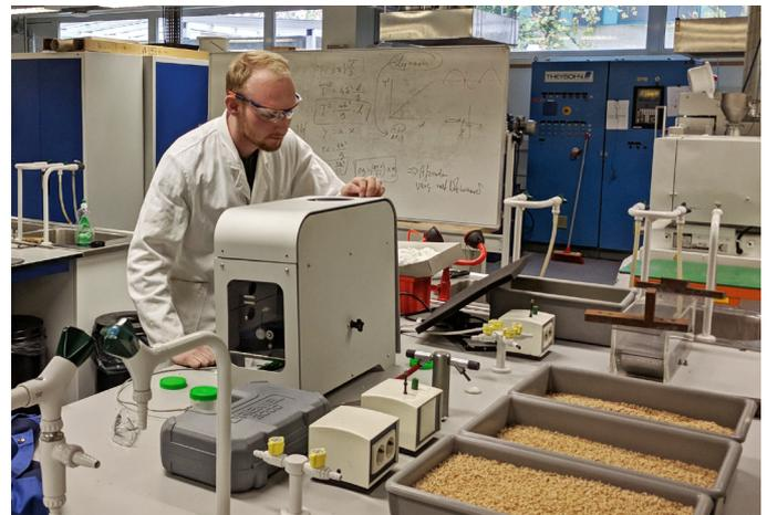
The NEXT being used to make small batches of material, as part of the polymer research projects by Fontys students.
